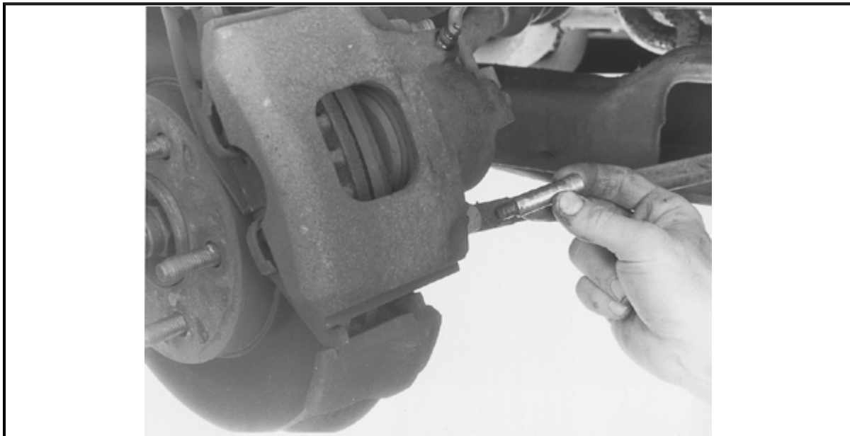
Removing one of two caliper locating pins
