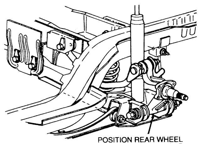
POSITION REAR WHEEL SPINDLE 4A013 IN REAR SUSPENSION ARM AND BUSHING 5500. INSTALL NEW BOLT, WASHER, NUT AND ADJUSTING CAM. TIGHTEN NUT TO 54-71 N·m (40-52 LB-FT)
