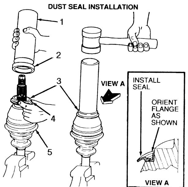
NOTE: CLAMP HALFSHAFT IN VISE AND INSTALL USING SPINDLE AXLE SEAL REPLACER T83T-3132-A1 AND FRONT BEARING DUST SEAL REPLACER T89P-1104-A4 WITH SEAL FLANGE FACING OUTBOARD.
