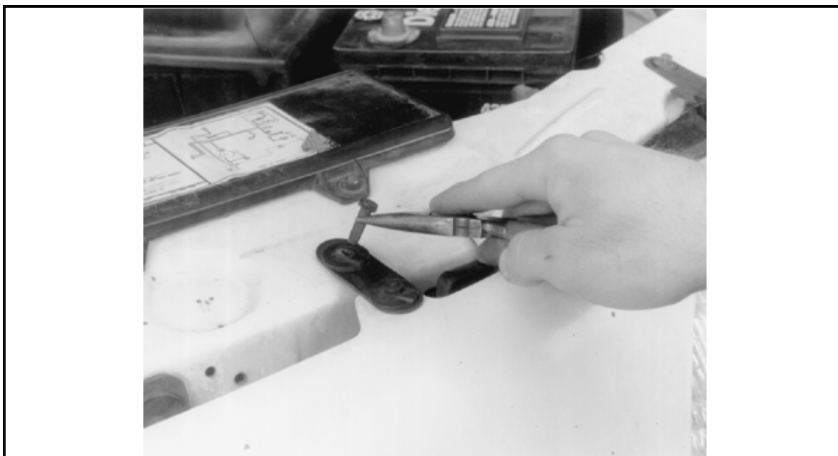
On Taurus, detach the grille retainers, then remove the grille
