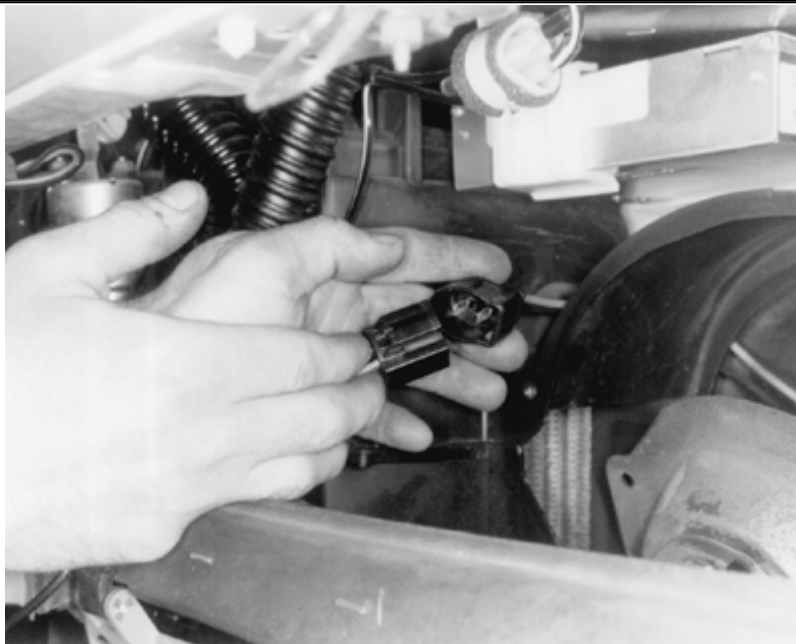
Disengage the electrical connector
