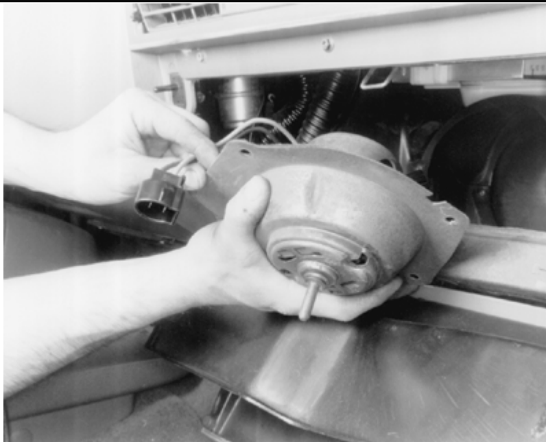
Remove the blower motor assembly from the vehicle
