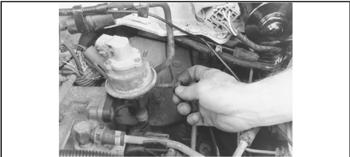
Remove the mounting bolts from the EGR valve
