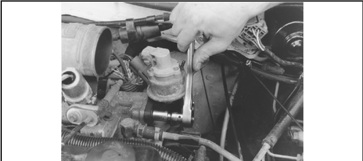
Disconnect the mounting bolts from the EGR valve
