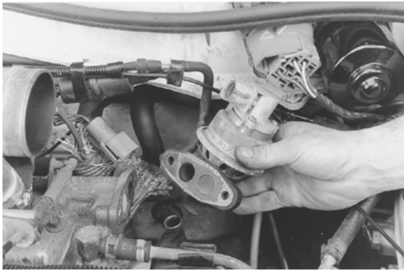
Remove the EGR valve from the vehicle-early model engine shown
