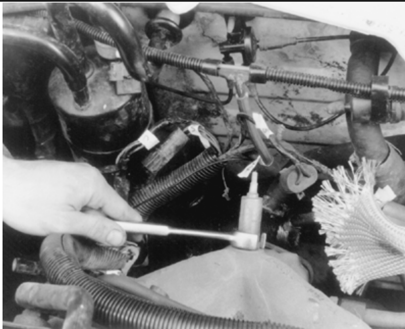
After disengaging the electrical connector, unscrew the heated oxygen sensor-2.5L engine shown
