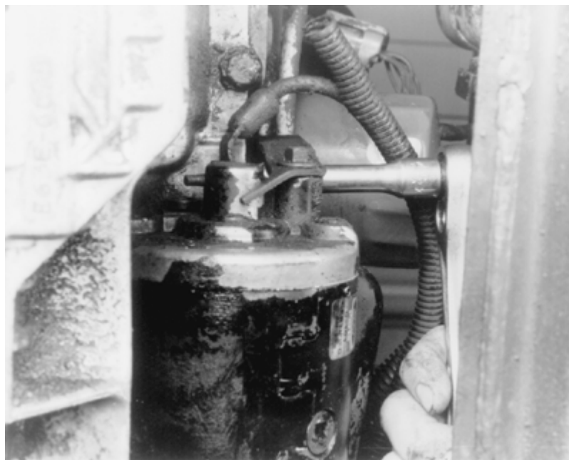
Remove the starter retaining bolts-early model 2.5L shown
