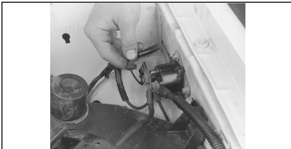
Disengage the relay-to-ignition switch electrical connector-early model 2.5L shown
