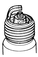
IDENTIFIED BY BLACK, DRY FLUFFY CARBON DEPOSITS ON INSULATOR TIPS, EXPOSED SHELL SURFACES AND ELECTRODES.
