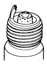
IDENTIFIED BY MELTED ELECTRODES AND POSSIBLY BLISTERED INSULATOR. METALIC DEPOSITS ON INSULATOR INDICATE ENGINE DAMAGE.
