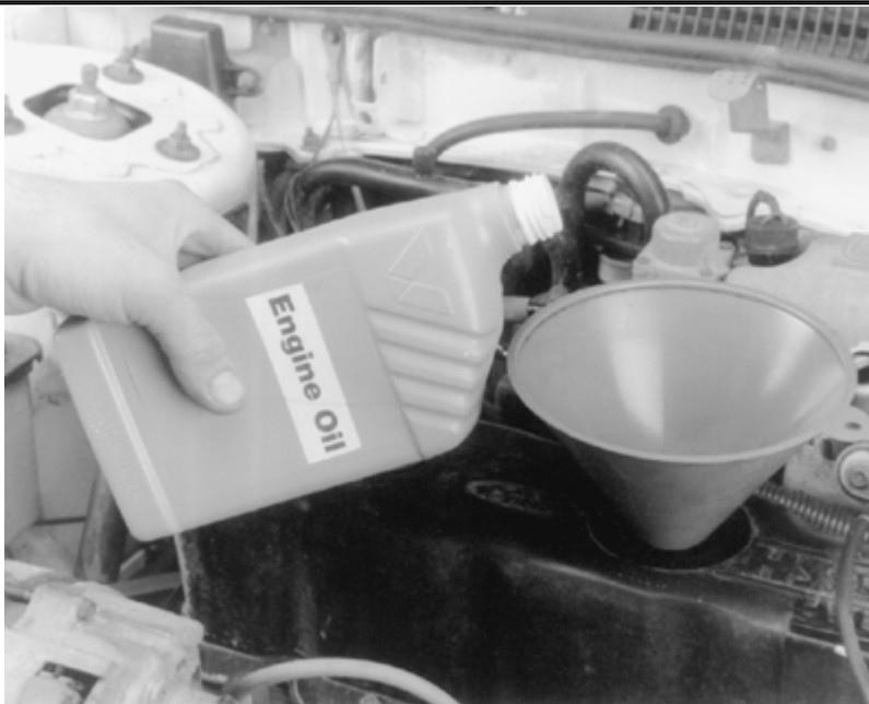
Refill the crankcase with the proper grade and capacity of engine oil
