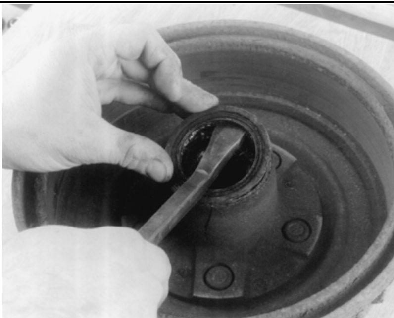
Removing the grease seal; discard the seal after removing. Note that the preferred method for removing the seal is with a proper seal remover tool
