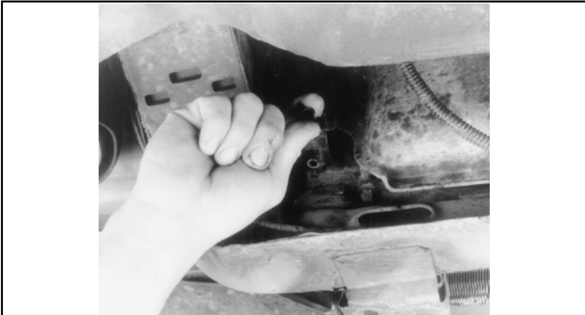
Open the drain valve located on the bottom of the radiator
