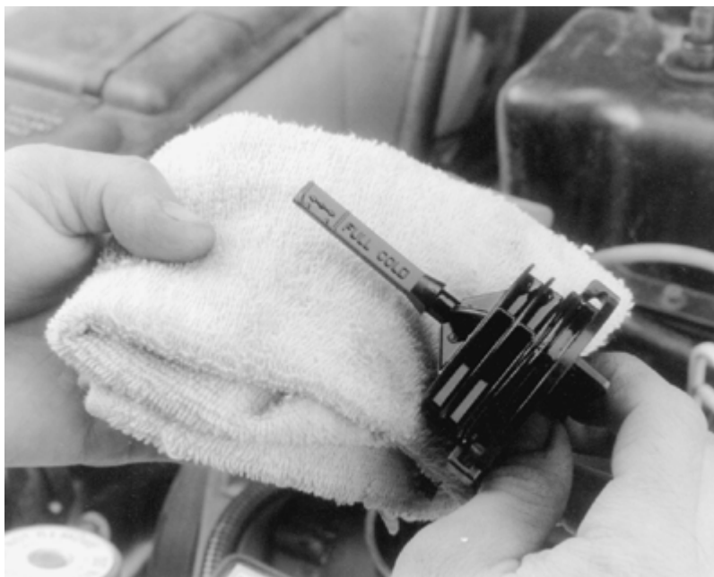
Power steering dipstick fluid level marks for checking the fluid when the engine is cold
