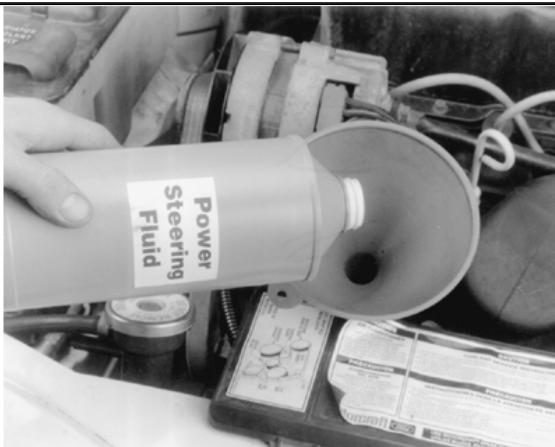
Add power steering fluid in small amounts, but do not overfill
