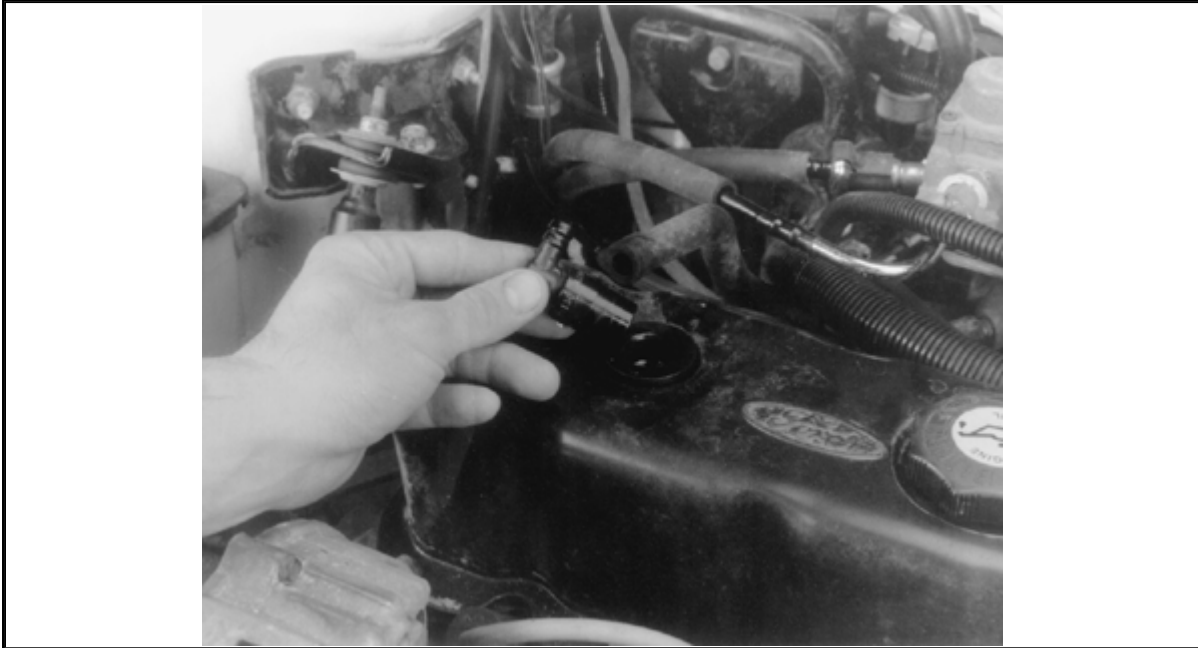
PCV system-early model 2.5L engine shown
