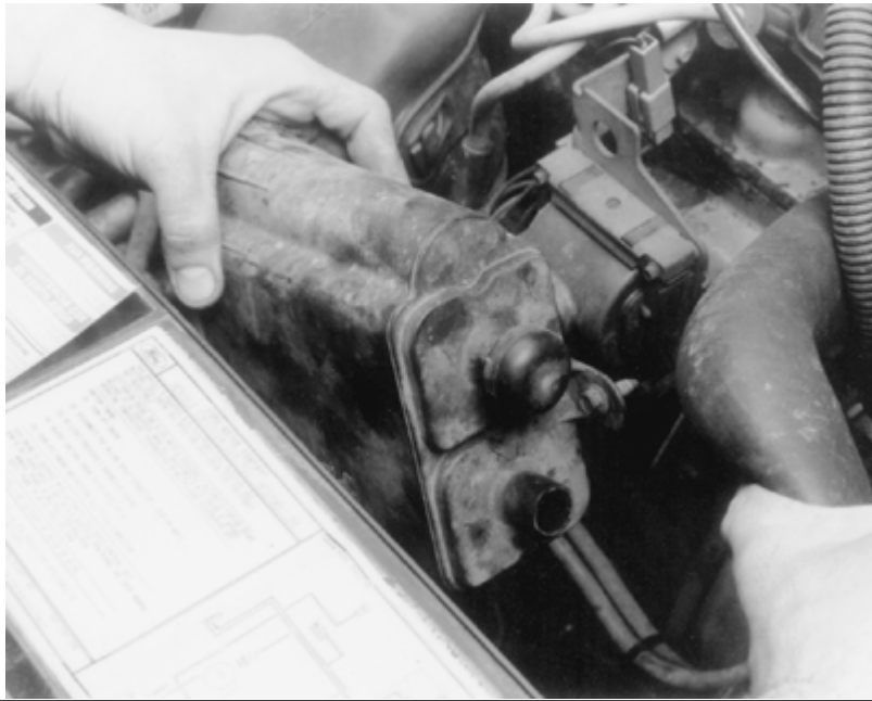
Removing the carbon canister-Early model 2.5L shown
