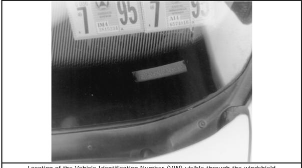
Location of the Vehicle Identification Number (VIN) visible through the windshield
