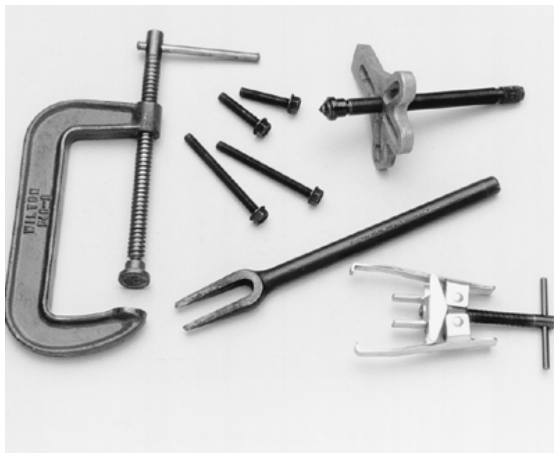
Various pullers, clamps and separator tools are needed for the repair of many components
