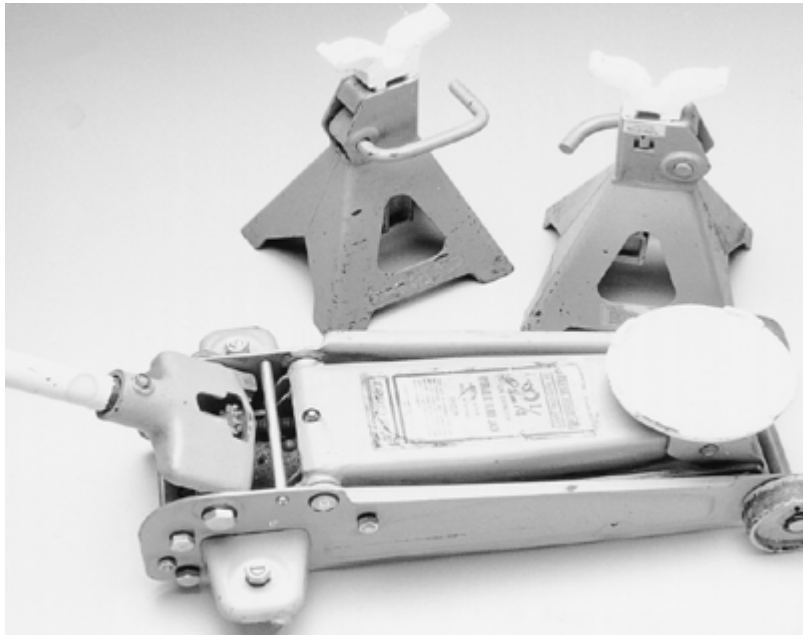
A hydraulic floor jack and a set of jackstands are essential for lifting and supporting the vehicle
